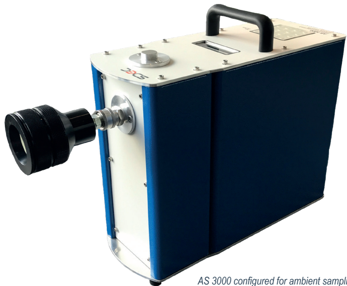
AS 3000 configured for ambient sampling (sampling on horizontal axis)
